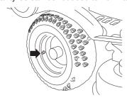
**IMPORTANT INFORMATION** Different tyre pressures on the front tyres will result in the blades cutting the grass at different heights. Having the same air pressure in the tyres is important in order to achieve the best possible performance as well as to avoid damage to the machine
